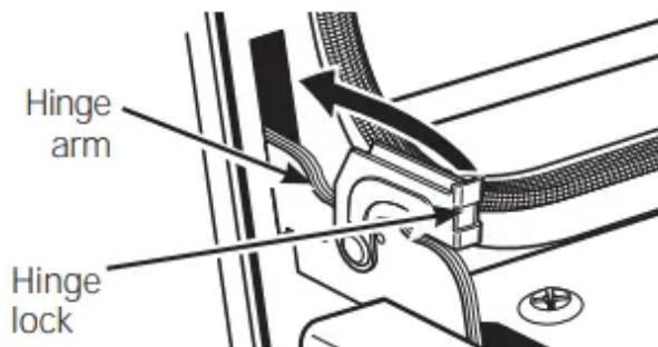
Push hinge locks up to lock
