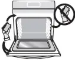
Figure 21: Clean around the oven door gasket
