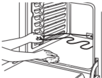
Gently lift the bake element
