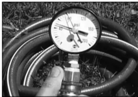
Figure 4 - Use a Water Pressure Gauge to make sure your home's water pressure is not too high.
