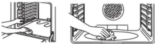
Gently lift the bake element Wipe up heavy soil on the oven bottom.
