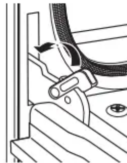
Push hinge locks down to lock
