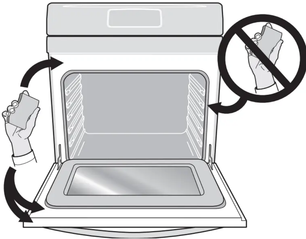
Figure 19: Clean around the oven door gasket
