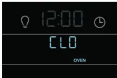
Figure 28: Message of open door that must be closed before oven can begin the clean cycle
