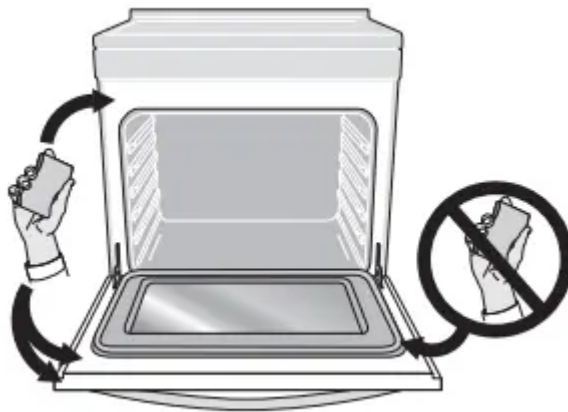
Figure 27: Areas to clean and areas to avoid (gasket)
