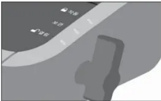
Close and turn Easy Lock Latch to OPERATE position
