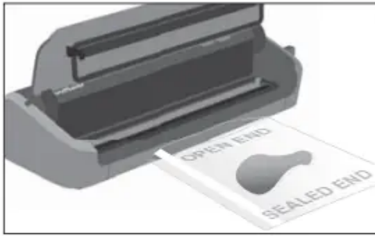
Place Bag in Vacuum Channel
