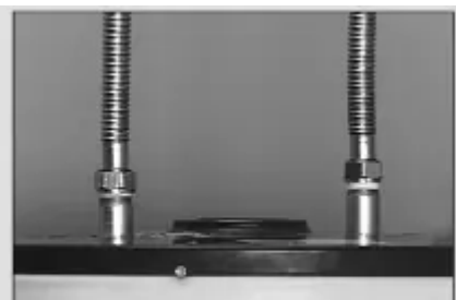
Compression fittings don't require soldering.
