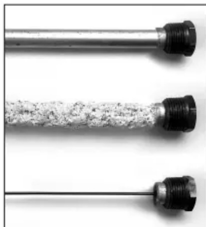
Figure 43 - Anode rods from new (top) to partially depleted (middle) to fully depleted stage (bottom).
