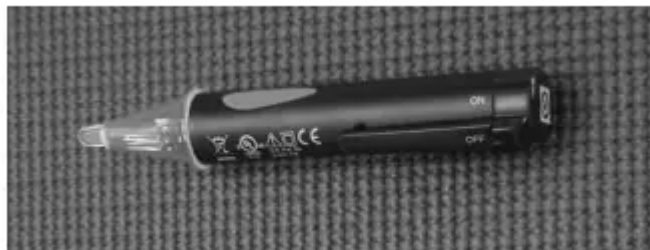
Figure 21 - Use a non-contact circuit tester to check for electrical power.
