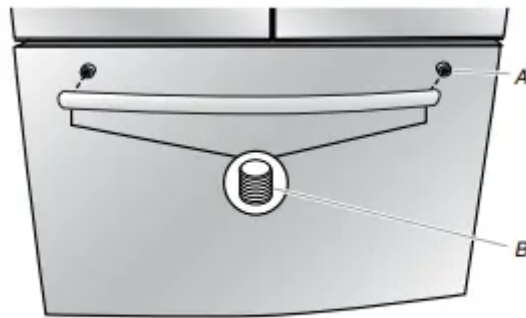
A. Shoulder screw B. Setscrews inside the handle
