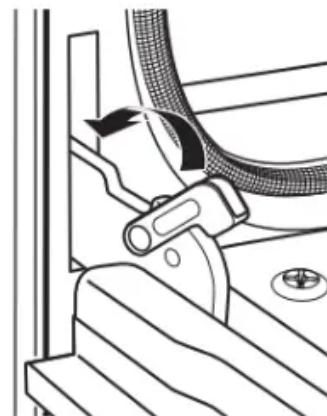
Push hinge locks down to lock
