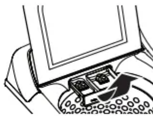
GTW680 and GTW685 models have a large dispenser drawer with compartments for both detergent and softener.
