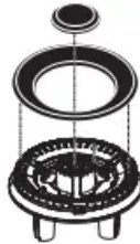
Multi-Ring Burner (on some models) Use this burner for large cookware or for simmering applications.
