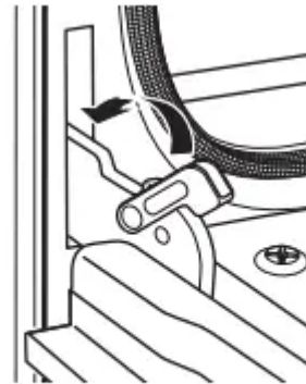
Push hinge locks down to lock
