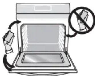
Figure 19: Clean around the oven door gasket
