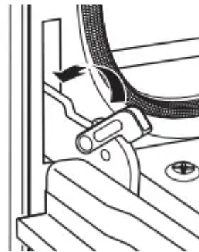
Push hinge locks down to lock
