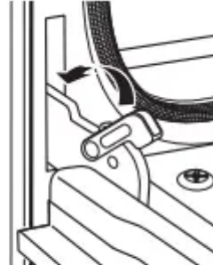
Push hinge locks down to lock
