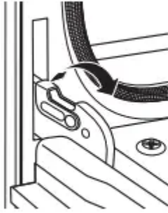
Pull hinge locks up to unlock
