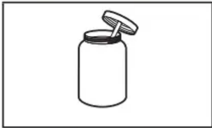
Pipe-joint compound resistant to propane gas
