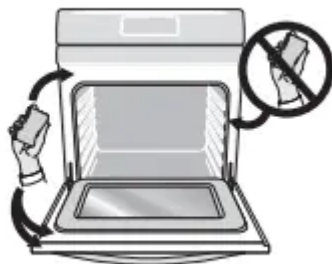
Figure 19: Clean around the oven door gasket
