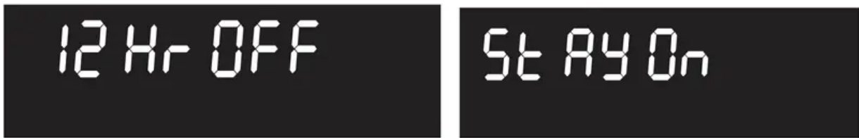
Figure 22: 12 hr energy saving (L) and continuous setting (R)
