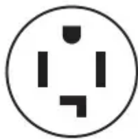
4-wire receptacle (14-30R)
