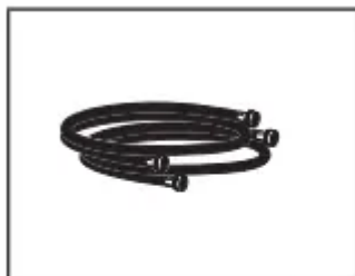
Inlet hoses with flat washers
