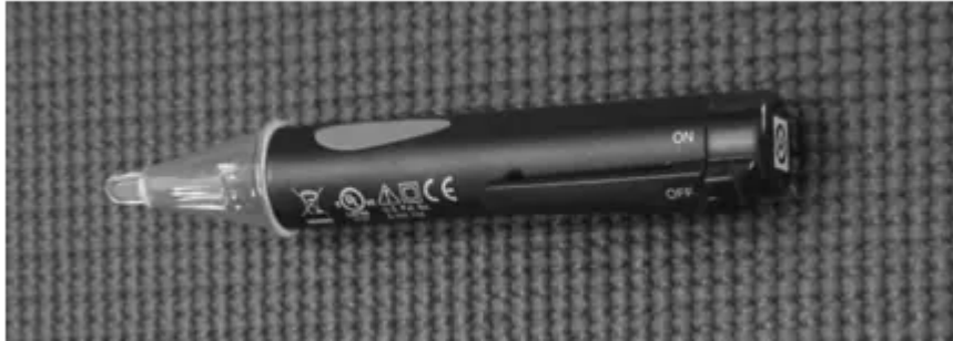
Figure 28 - Non-Contact Circuit Tester
