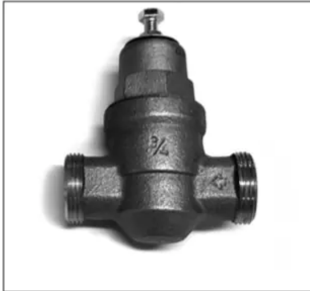
Figure 15 - A Pressure Reducing Valve is required if your home's water pressure is above 80 psi.
