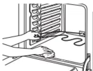
Gently lift the bake element
