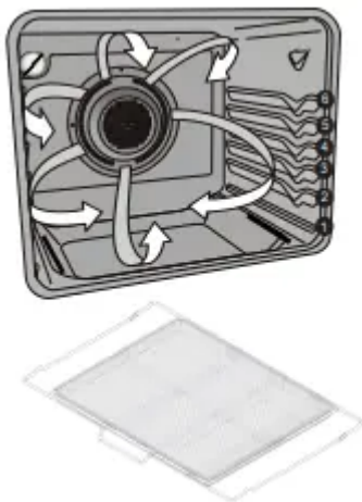
Figure 25: Optional Frigidaire Air Fry Tray. Use rack position 3 with tray or dark pan with low or no sides for best results.
