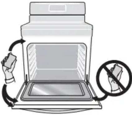
Fig. 33 Areas to clean and areas to avoid (gasket)
