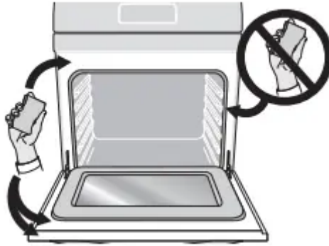
Figure 27: Clean around the oven door gasket
