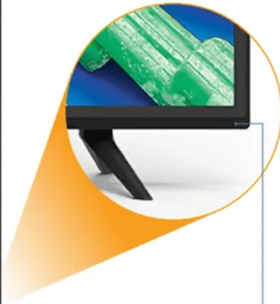
Remote Sensor and Power Indicator When using the remote, aim it directly at this sensor. The power indicator flashes on when the TV turns on, then goes out after several seconds. To keep the power indicator on, see Turning the Power Indicator On or Off on page 23.
