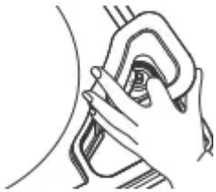
Fig.26 Removing the Wash Boost funnel
