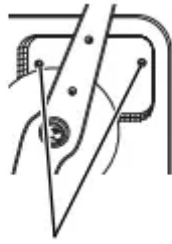
Sump cover screws
