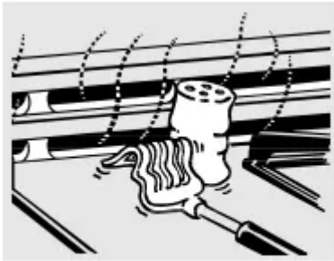
Plastic items on the cooktop may melt if left too close to the vent.
