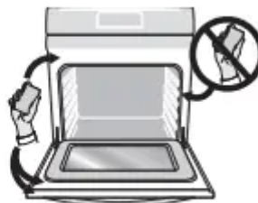
Figure 23: Clean around the oven door gasket
