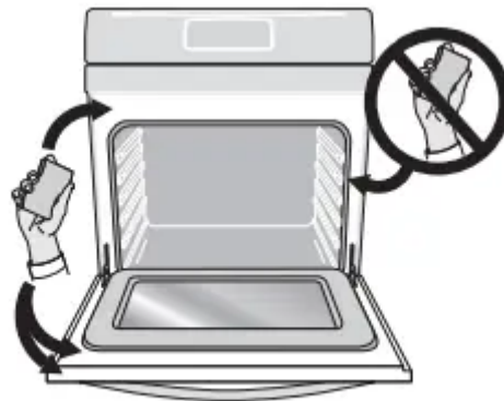
Figure 21: Clean around the oven door gasket
