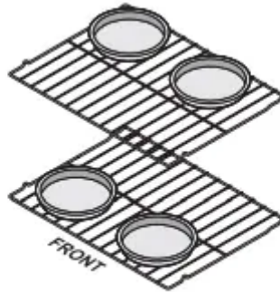
Figure 16: Pan positions two rack baking
