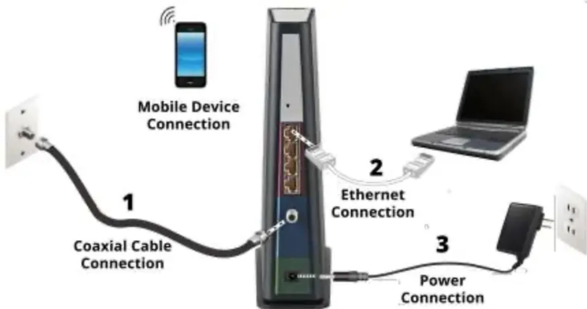
Figure 4: SBG8300 connection diagram
