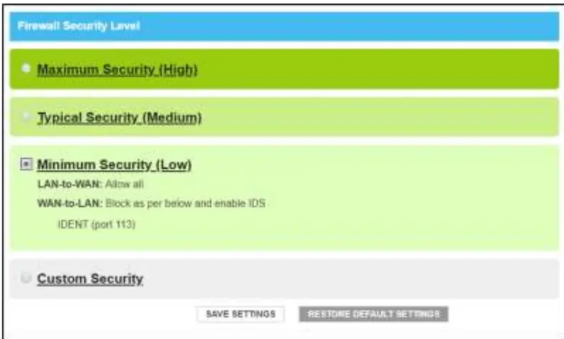
Figure 39: Firewall IPv4 low security level screen
