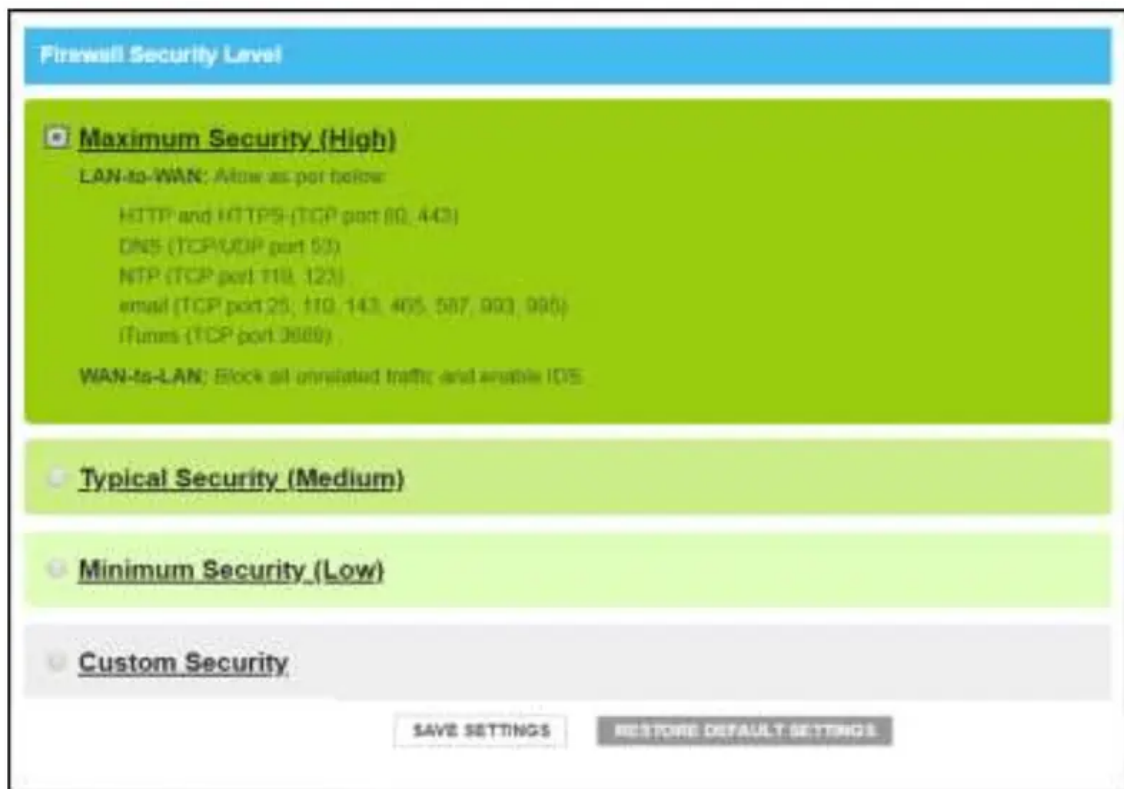
Figure 37: Firewall IPv4 high security level screen
