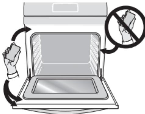
Figure 24: Clean around the oven door gasket
