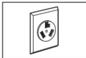
3-wire receptacle (NEMA type 10-30R)
