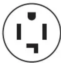
4-wire receptacle (14-30R)
