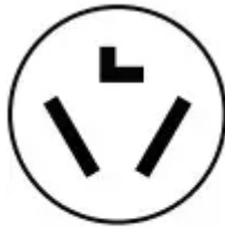
3-wire receptacle (10-30R)
