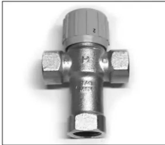
Figure 20 - Adjust Thermostat Mixing Valves at each point-of-use 120°F or lower.
