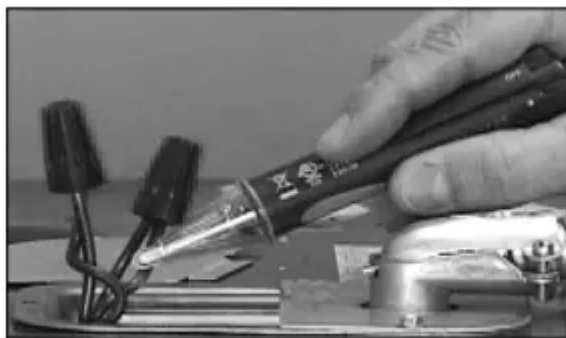
Figure 37 - Non-Contact Circuit Tester
