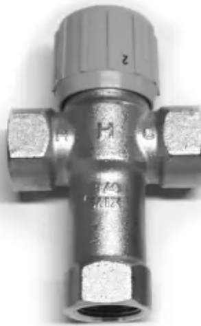
Figure 7 - Thermostatic Mixing Valves installed at each point-of-use can help prevent scalds.
