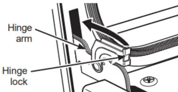
Push hinge locks up to lock
