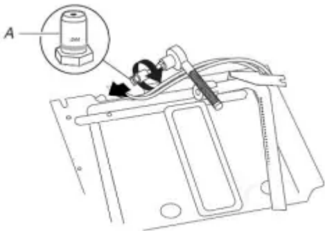
A. Number 0.044 Propane gas orifice hood
