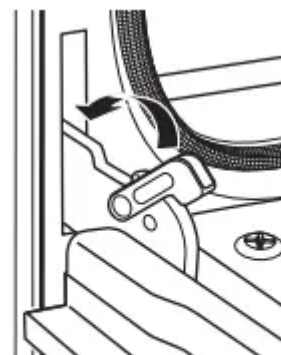
Push hinge locks down to lock
