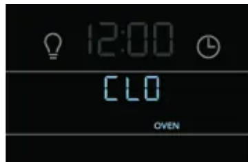
Figure 28: Message of open door that must be closed before oven can begin the clean cycle
