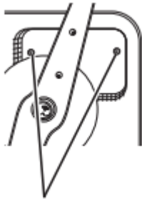
Sump cover screws
