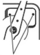
Sump cover screws
