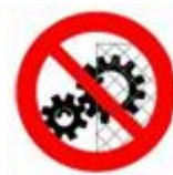
Prohibition to remove the safety devices and guards
