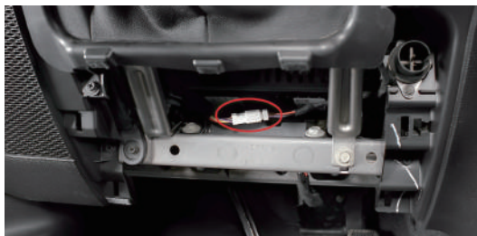
5.4 Run the wire harness behind the dash.
