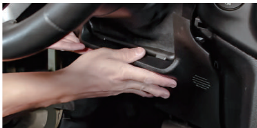
5.6 Put the black plastic panel back on.
