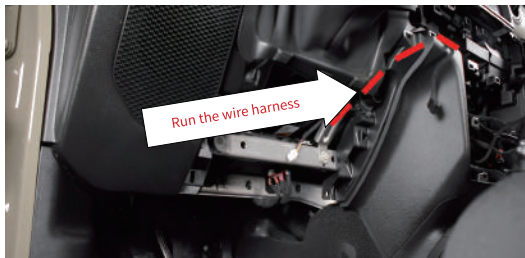
5.5 Connect to the relay harness and ziptie it.
