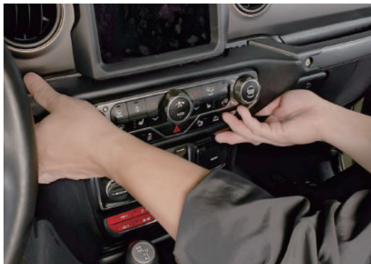
6.2 Put the top panel back on.
