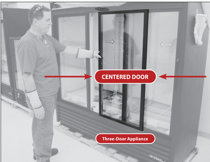
Fig. 3. Center the middle door on the right door's left edge.
