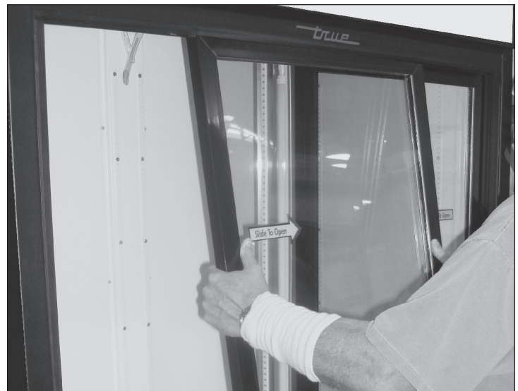
Fig. 4. Carefully remove the door.
