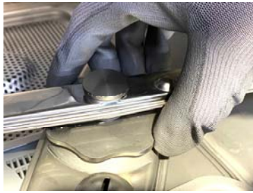
Daily disassemble the lower and upper rinse arms by working on the „big“ ring nut, like in the picture.
