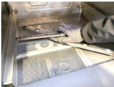
Unscrew the lower rinse arm
