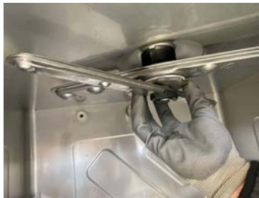
Remove the rinse arm on the top
