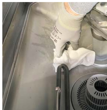
Remove from the tank by means of a brush or cloth if any, residual dirt.
