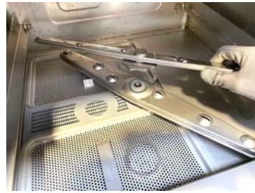
Remove the lower rinse arm
